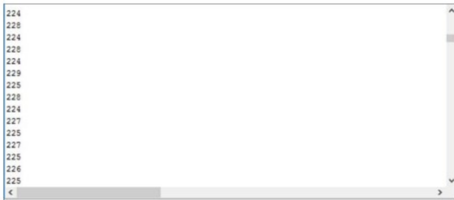
Fig. 1.3 : The reading shown on Serial Monitor when the LDR sensor board is being exposed to sunlight.
